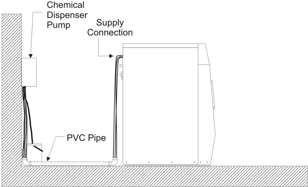
Figure 4.16: External Chemical Supply Connection Detail
