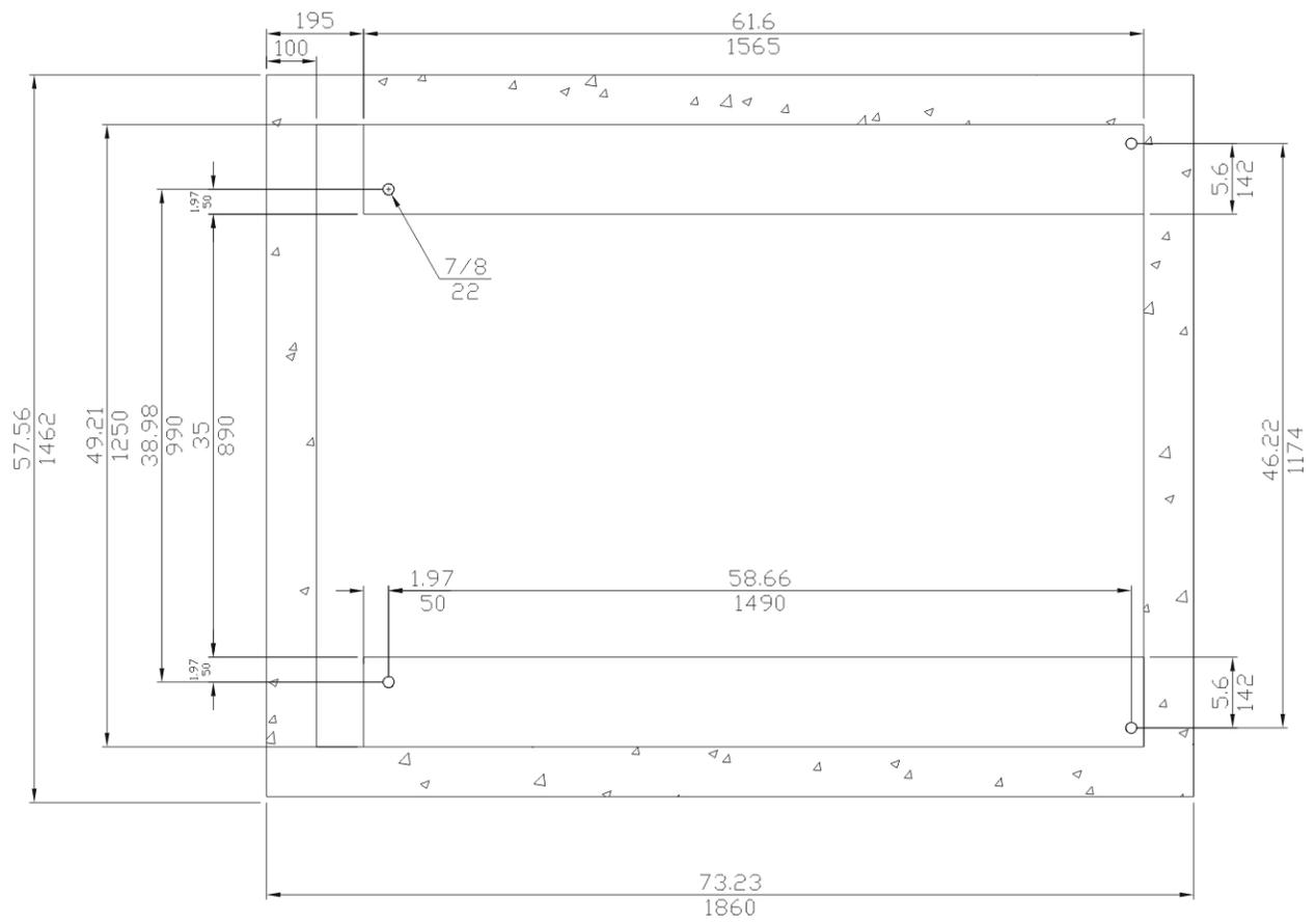
Figure 4.8: SP-155/165 Bolt Hole Layout
