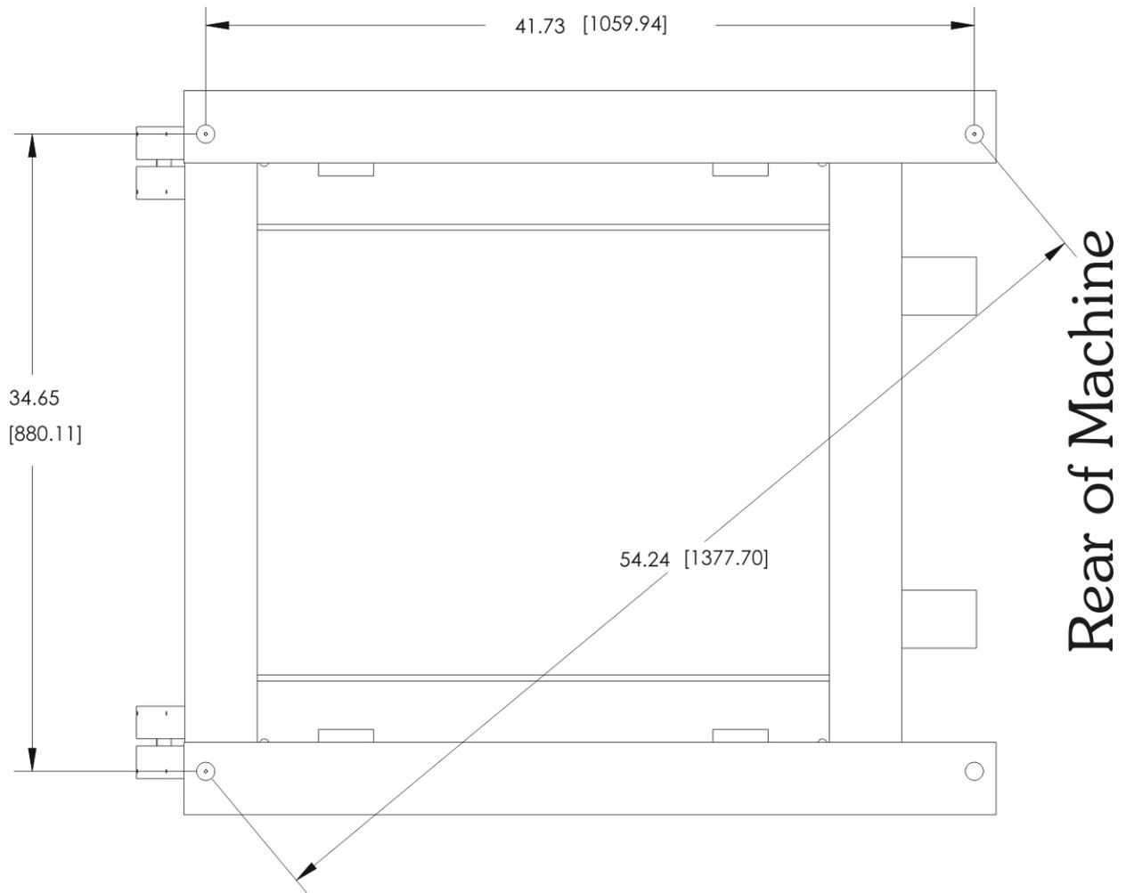
Figure 4.4: SP-60/65 Bolt Hole Layout
