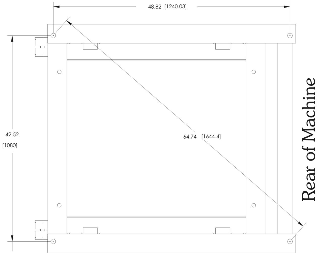
Figure 4.6: SP-100/110 Bolt Hole Layout
