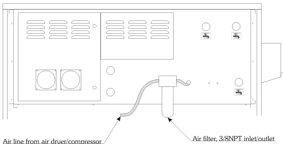
Figure 4.15: Compressed Air Connection Detail
