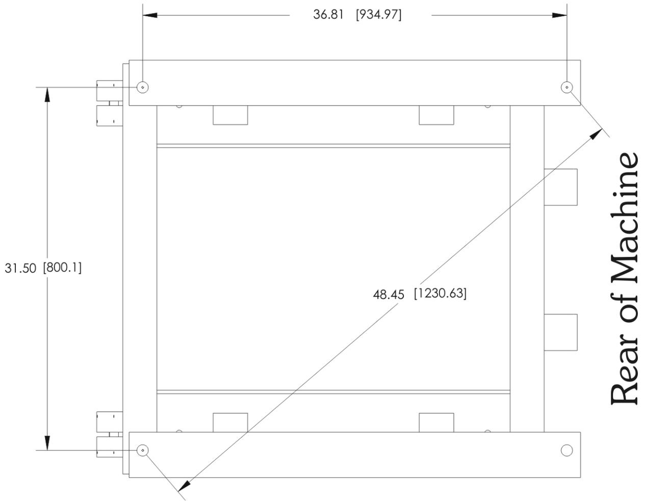
Figure 4.2: SP-40/45 Bolt Hole Layout
