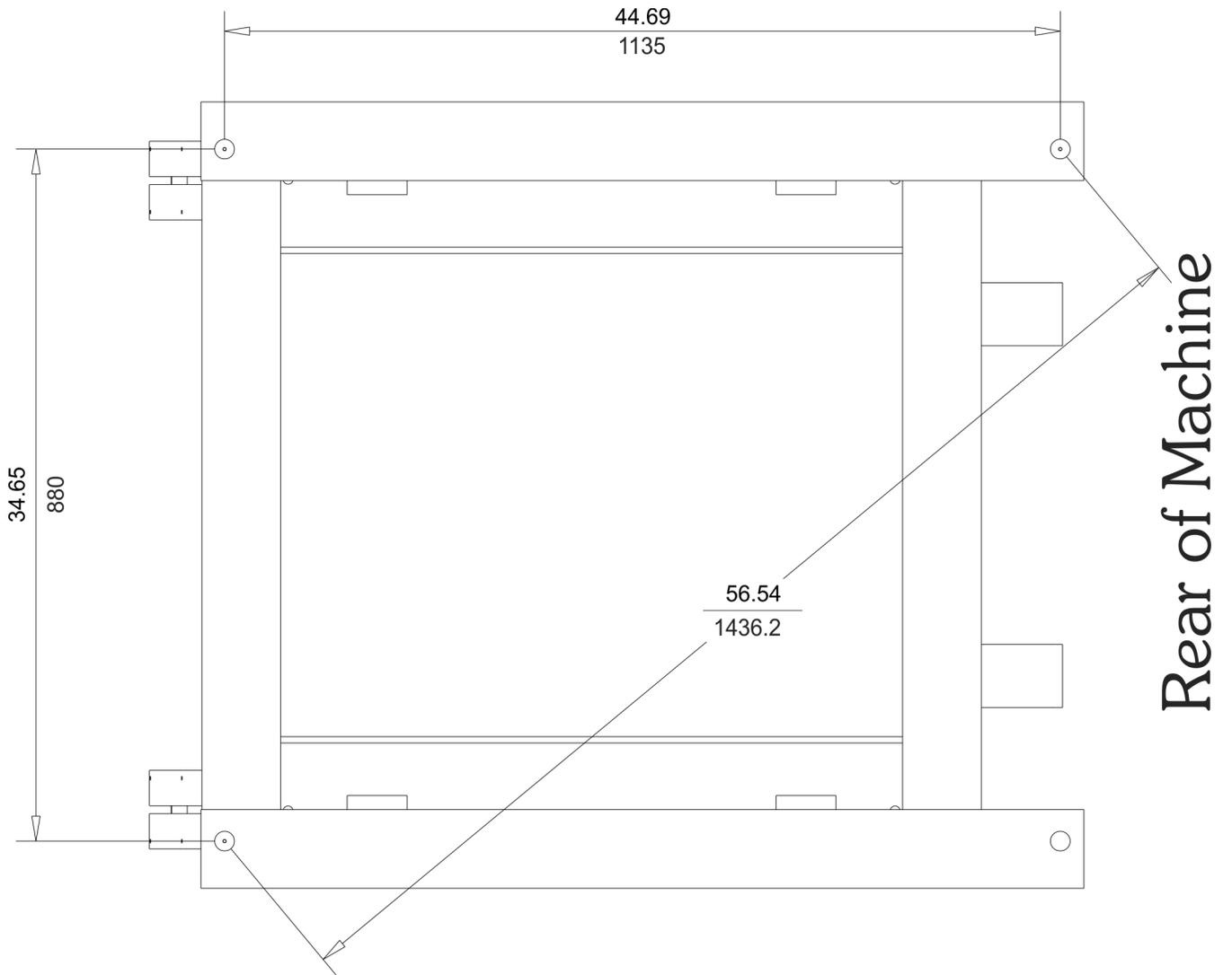
Figure 4.5: SP-75 Bolt Hole Layout
