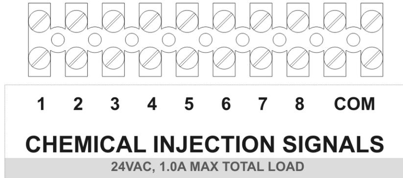
Figure 4.19: External Chemical Supply Terminal Block Detail
