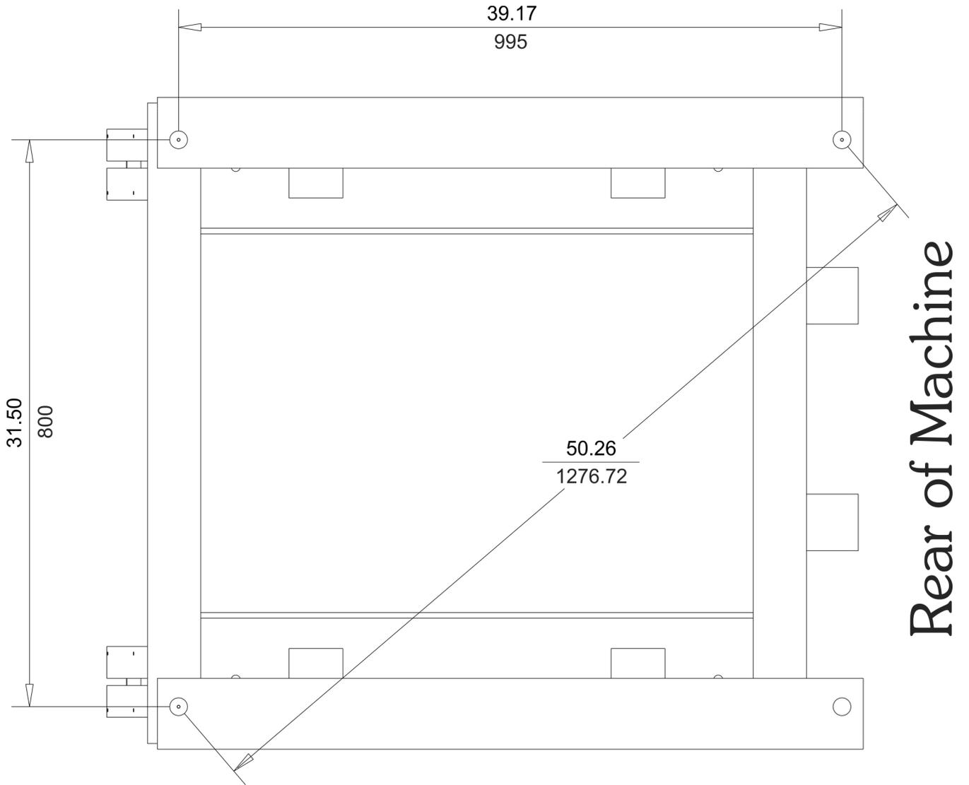
Figure 4.3: SP-50 Bolt Hole Layout
