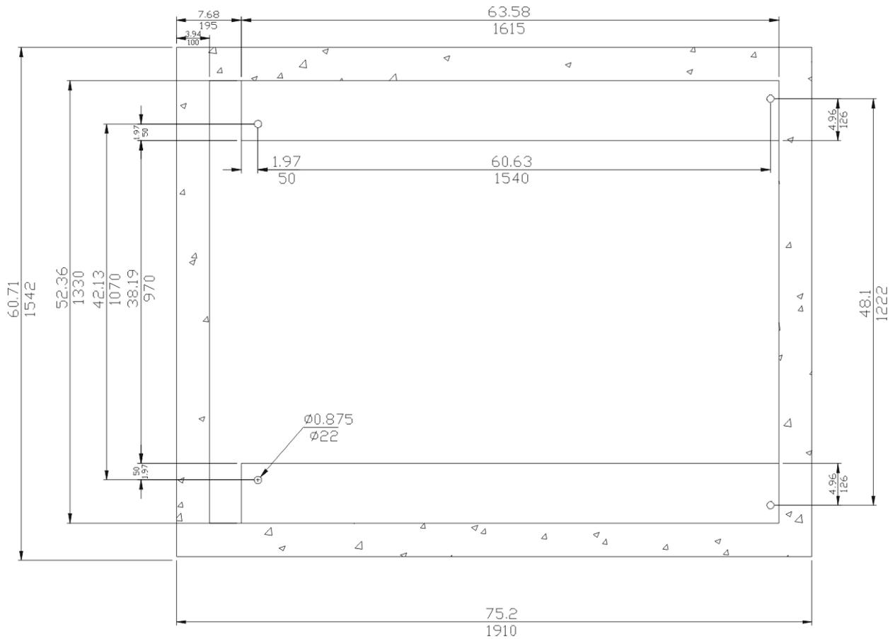
Figure 4.9: SP-185/195 Bolt Hole Layout
