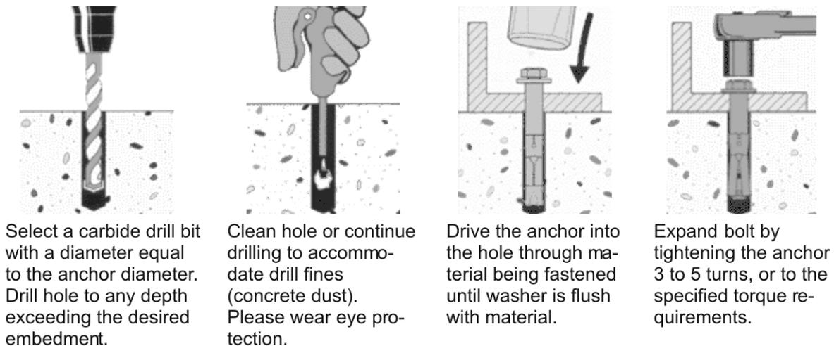
Figure 4.10: Typical Machinery Anchor Installation
