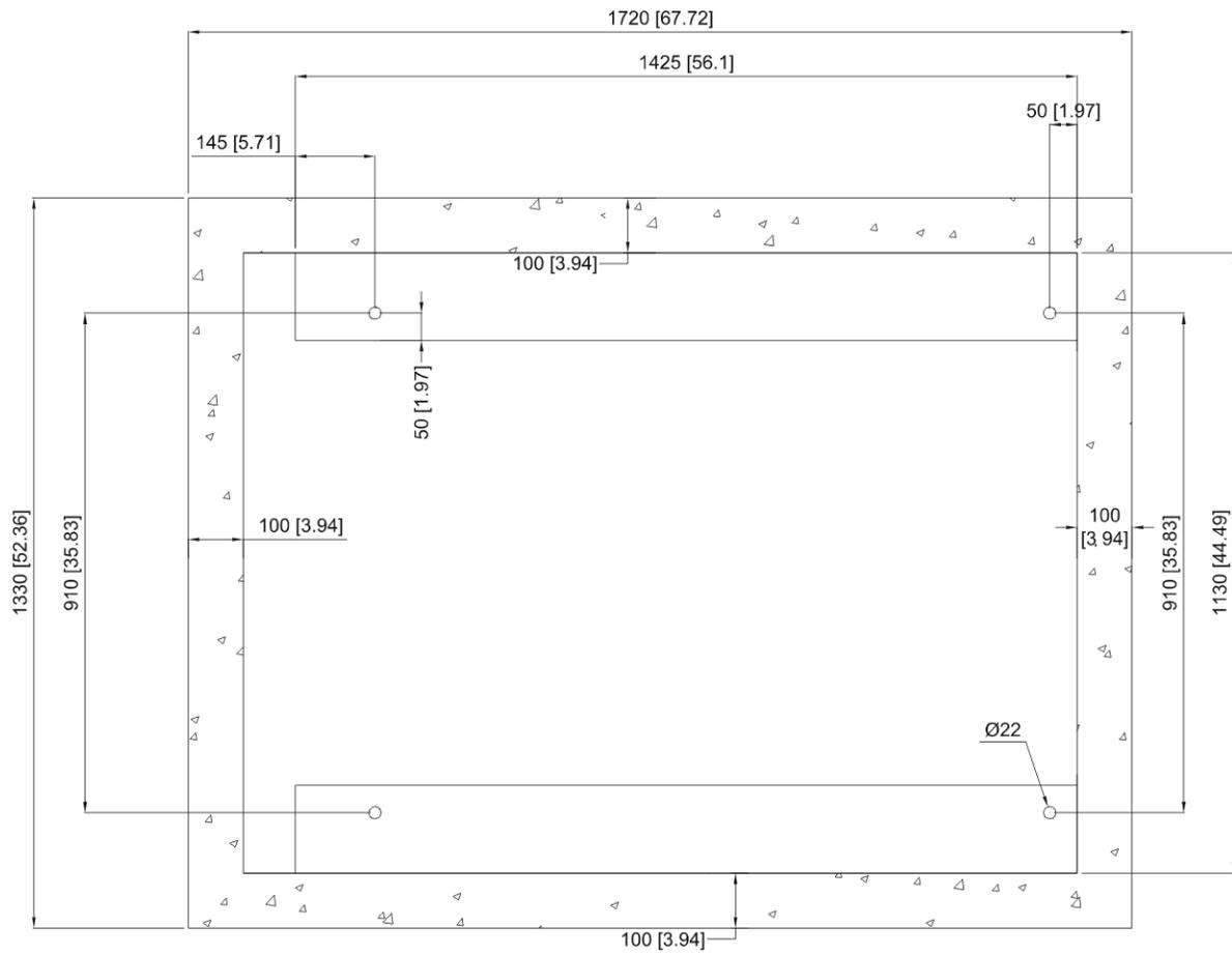
Figure 4.7: SP-130/135 Bolt Hole Layout
