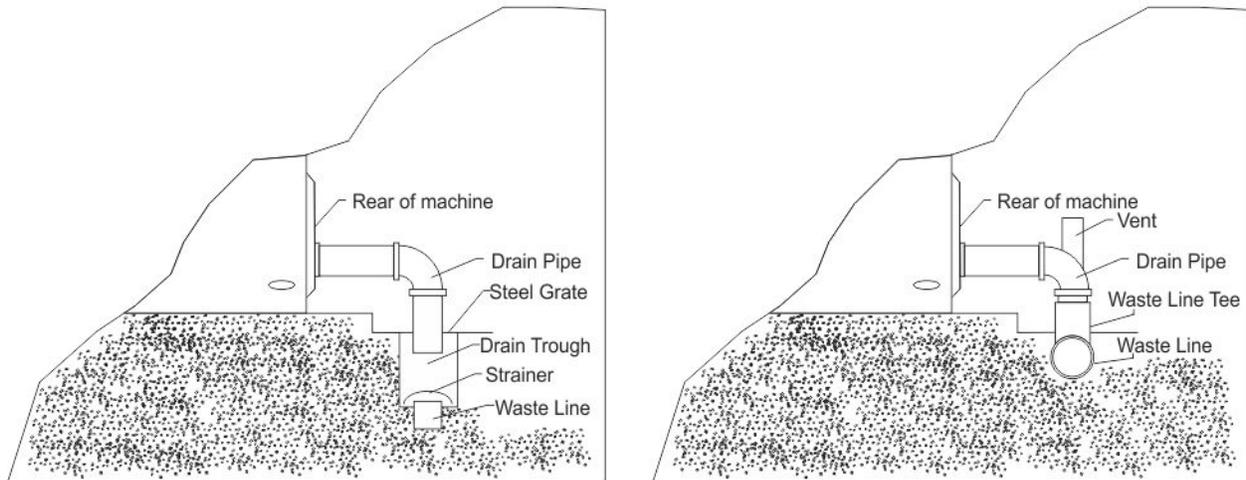
Figure 4.12: Drain System Information
