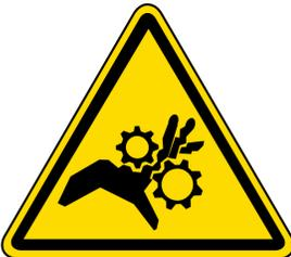
This warning symbol alerts you to the presence of possible dangerous drive mechanisms within the machine. Guards should always be in place when the machine is operation. Be careful when servicing any drive mechanism.
